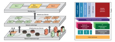
Network slicing calls for a novel architecture capable of flexibly orchestrating and configuring all the resources, functions, and entities used by a network slice  $\rightarrow$  Network softwarization
