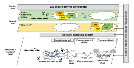
Aim: Architecture flexibility, heterogeneous accesses, vertical business integration Enablers: SDN; NFV; Modularization; Network Slicing; Network
